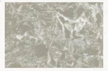
Made by mixing natural marble dust with resins, non-toxic chemicals and special pigments, composite marble blocks are cast, dried and cured naturally in the open, under the sun, sawn into slabs by gang saw machines. The slabs are then calibrated for thickness and polished on very high-tech line polishers.
